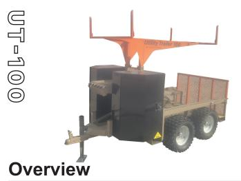
The InnovaTech Utility Trailer is designed to pull behind a small tractor or Side-by-Side on a jobsite. It has racks for ladders or materials, a bed capable of holding buckets or a pallet, two tool cabinets, and two tool/work shelves, and a row of tool slots for hammers, screw drivers, or wrenches. The trailer sits on four OHV tires for use inside or outside of construction buildings.
